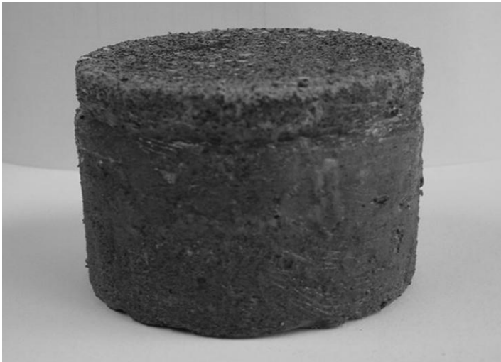
15.15 Multilayer sample with partially compacted clay inside it.
