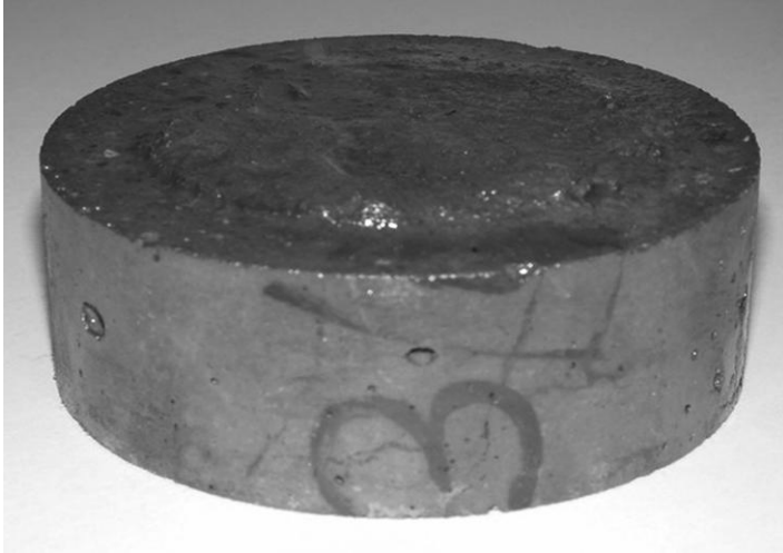
15.13 Cracked sample after clay has sealed the cracks.
