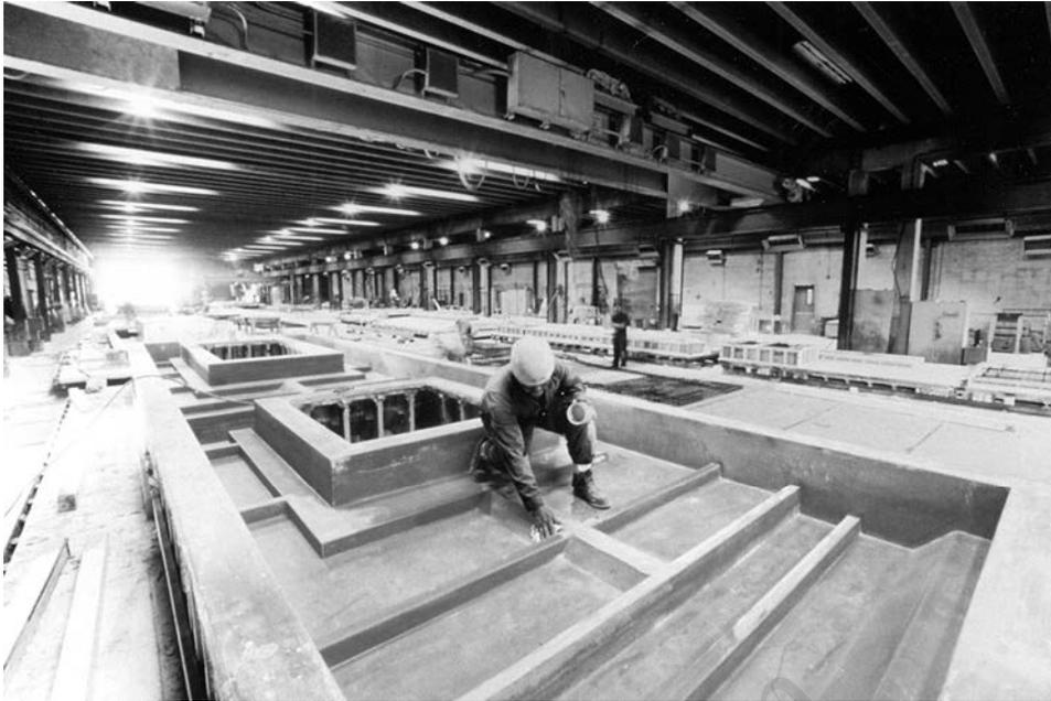
Fig. 6.2.1(a)—Mold for casting precast panel.
