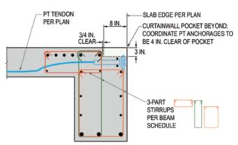
Fig. 4: The spandrel beam reinforcing was coordinated with curtainwall anchor pockets and PT tendon anchorages (Note: 1 in. = 25.4 mm)
