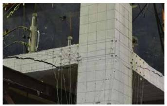
Crack pattern in corner slab-column connection at 1.25% drift (Fig. 4.43 from Final Report to the ACI Foundation: CRC 80)
