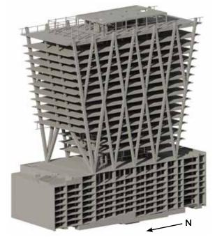
office building Fig. 1: The building structure features a unique lateral system consisting nediately of a diagonalized, architecturally exposed concrete exoskeleton
