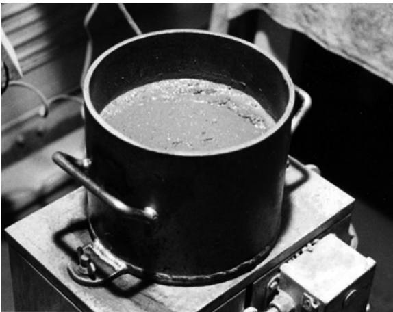
Fig. 7.2—Vebe consistency test time with ring of mortar on consolidated sample. (Photo courtesy of U.S. Bureau of Reclamation, 1985.)
