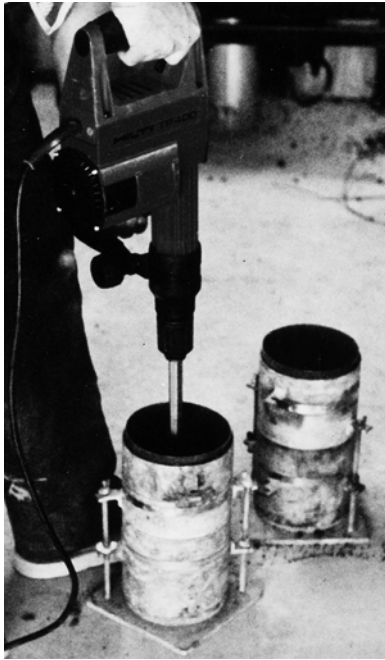
Fig. 7.5—Making RCC test cylinders with vibrating hammer.
