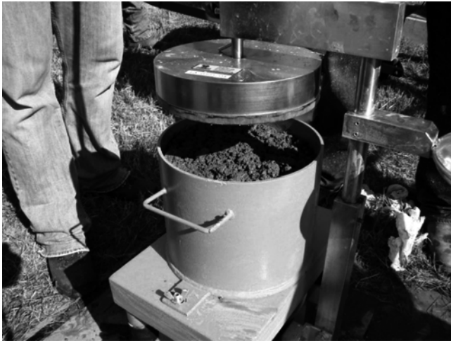
Fig. 3.1—ASTM C1170 Vebe consistency test apparatus with 27.5 lb (12 kg) surcharge. (Photo courtesy of U.S. Department of Agriculture, National Resources Conservation Service, 2008.)
