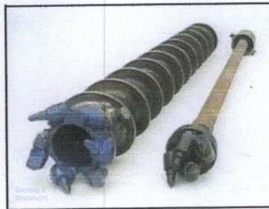
Figure 3-2. Hollow Stem Auger Components (ASTM D 4700).
