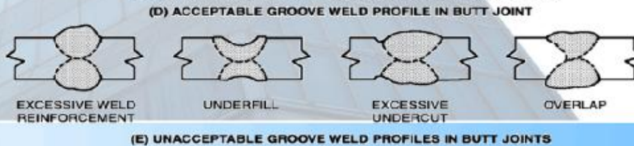
Figure 5.4—Acceptable and Unacceptable Weld Profiles (see 5.24)
