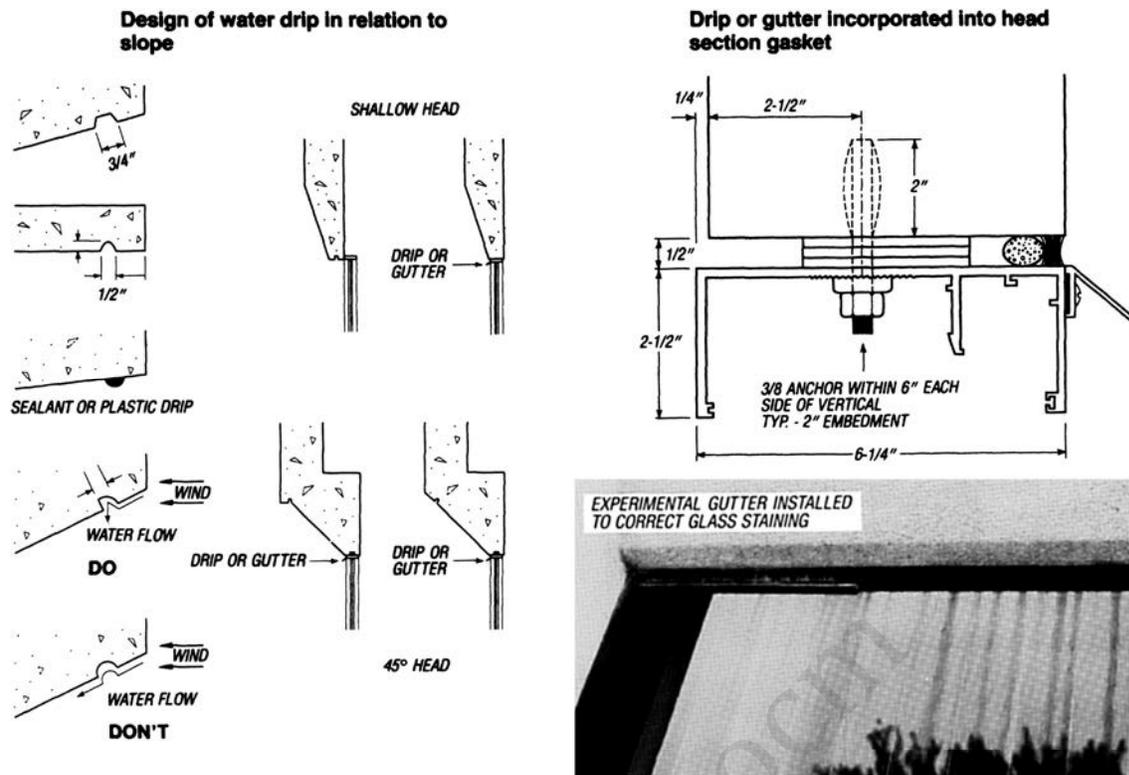
Fig. 3.7.1—Design of water drip in relation to slope.
