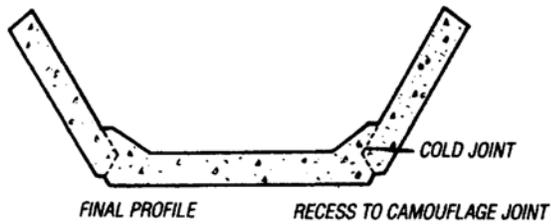
(a) separate casting stages of large returns
